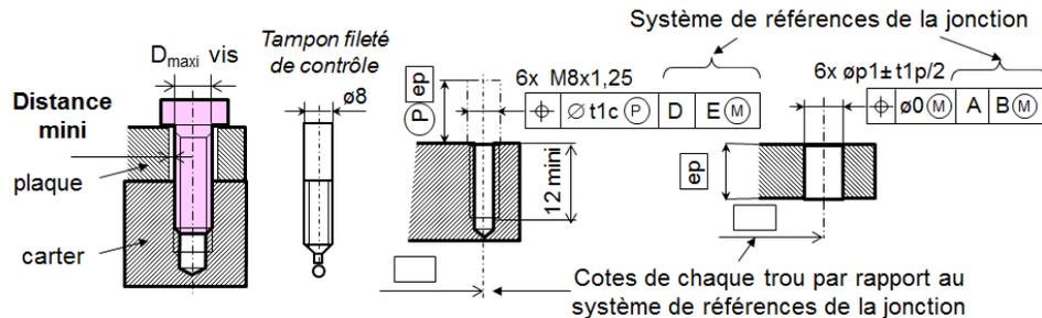
$$(p1 - t1p/2 - D_{maxi} \text{ vis} - t1c)/2 \geq \text{distance mini}$$
